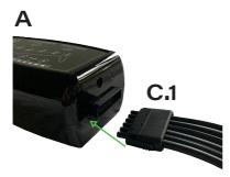
When assembling the machine, plug the Tube connector (C.1) into the control unit as demonstrated in the diagram.
