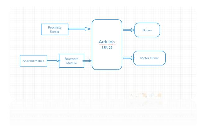
In this project, Arduino is interfacing with different hardware like a motor driver, HC05 Bluetooth Module, proximity sensor. When the sensor sense any metal body in ats range it creates an analog value by the respect of the distance between the sensor and metal body. Then the sensor sends the analog value into the Arduino board. Arduino also creates an Arduino pin which is connected with a buzzer. After detecting the metal, the buzzer will beep. For moving the motor we can remotely do it.
