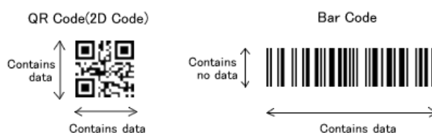
Figure 5. two-dimensional QR code vs one-dimensional barcode [9]
