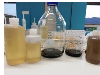
Figure 7: shows the washing process of graphene oxide
